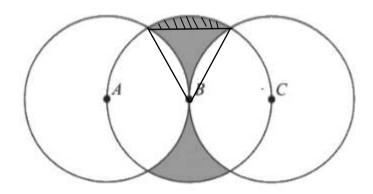
area of segment = area of sector centre B – area of equilateral triangle Total shaded area =  $2 \times (\text{area of sector} - 2 \times \text{area of segment})$ or  $2 \times (\text{area of triangle} - \text{area of segment})$
